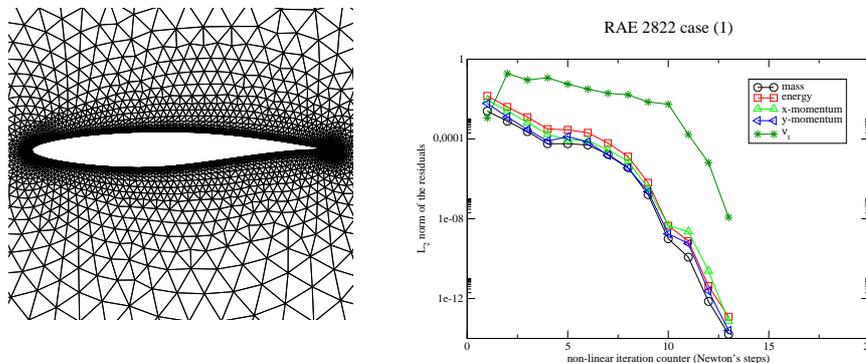
(a) Computational mesh for the RAE2822 (b)  $L_2$  residual norms versus the Newton's iteration counter.
